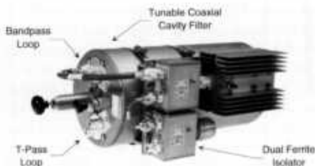
Figure 1 - Typical T-Pass Transmitter Multicoupler Channel Assembly
